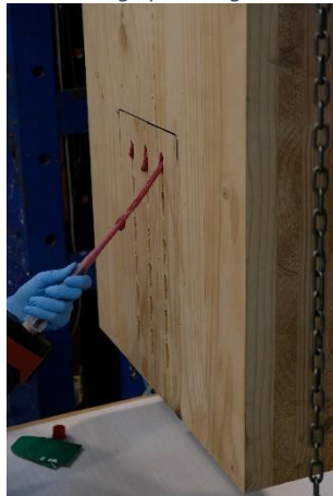
D – Injecting of epoxy
